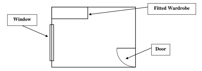
Here is the plan of a bedroom. It is drawn using a scale 2cm represents 1m.
